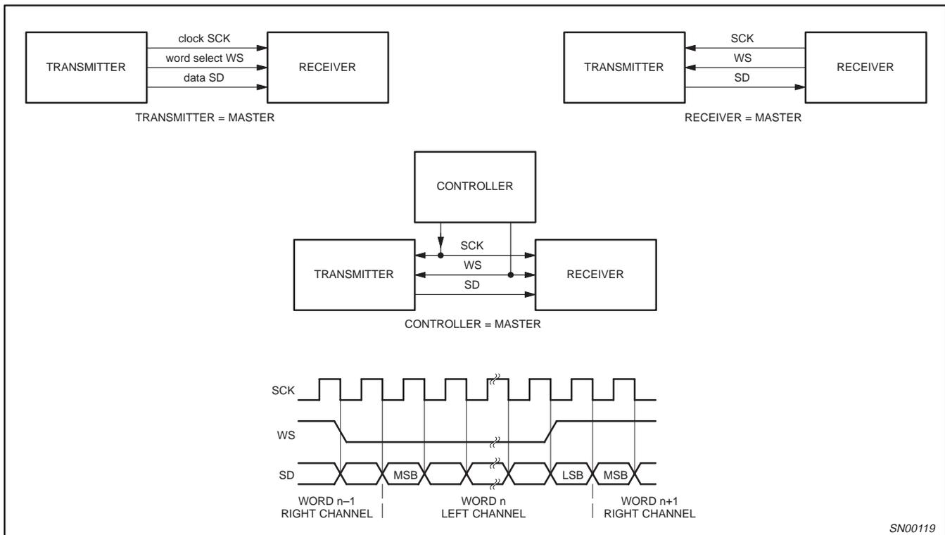
Figure 1. Simple System Configurations and Basic Interface Timing
