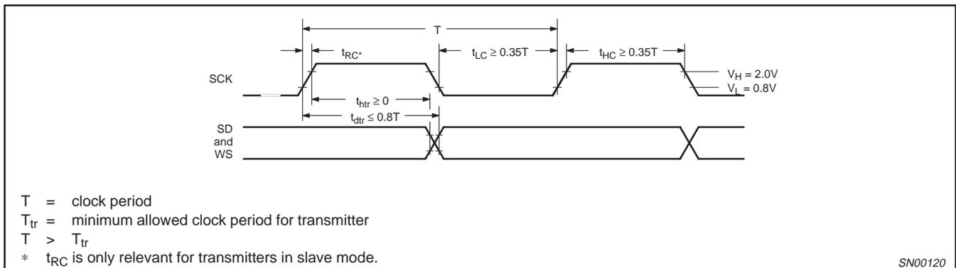
Figure 2. Timing for I<sup>2</sup>S Transmitter
