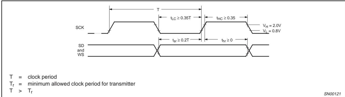
Figure 3. Timing for I<sup>2</sup>S Receiver
