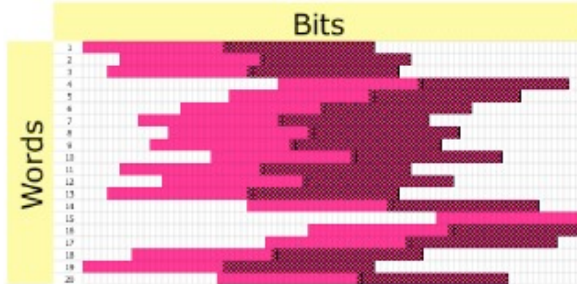
Figure 2.2 32-bit Floating-Point Data with Proposed Dither
